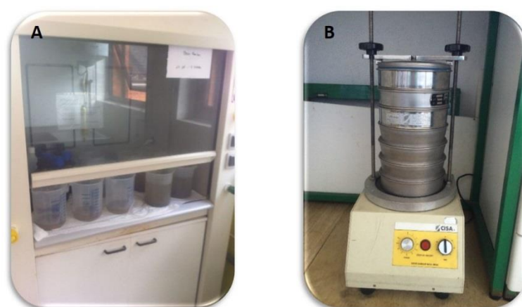
Figure 6. A- Destruction of organic matter with H_2O_2 ; B- Dry separation of sediments on a battery of sieves
