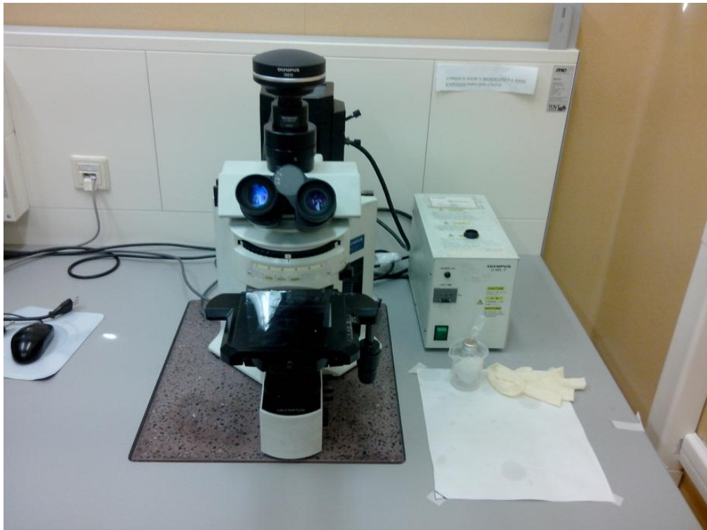
Figure 7: Epifluorescence microscope Olympus BX51, equipped with an Olympus XM10 camera
