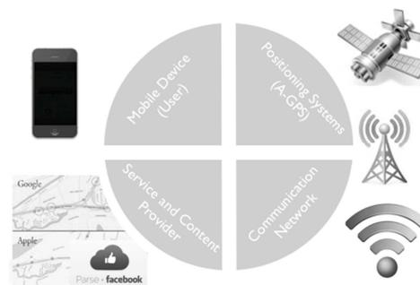
Figure 1. Four key basic components of any LBS
