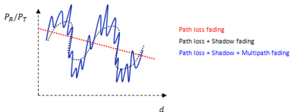
Figure 2. 1 - Power variation due path loss, shadowing and multipath
