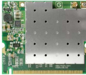
Figure 4.1: Wi-Fi Module containing 802.11p/DSRC Standard [83]
