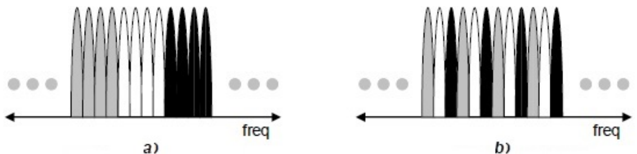
Figure 3.15: SC-FDMA sub-carriers mapped in Localized (a) and Distributed Mode (b) (Source: [35])
