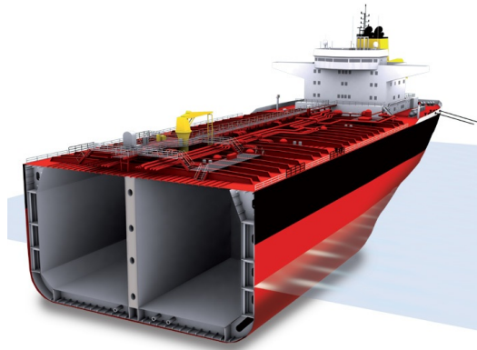
Figure 1.7: Principle structure of a double-hull tanker.
