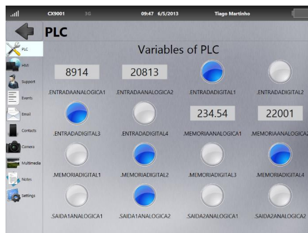
Figure 70 - Access the PLC: Create HMI Screen Implementation
