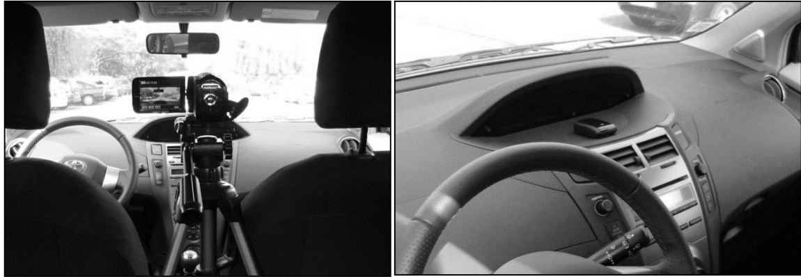
Figure 7 Scheme used for routes videotaping and GPS data logger location
