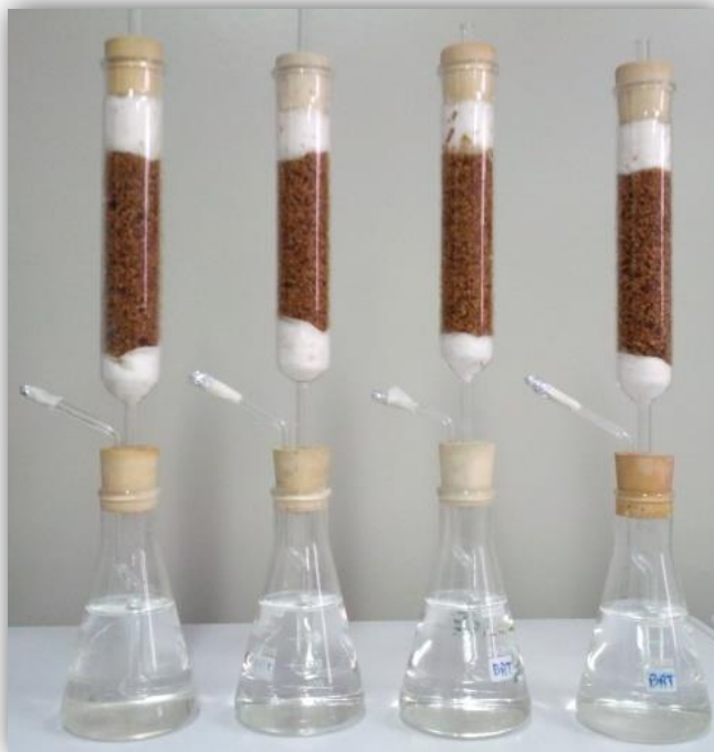
Figure 5 – Fixed bed column bioreactors for SSF containing inoculated orange peel.
