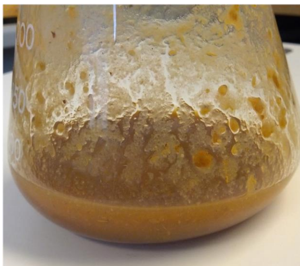
Figure 6 – Non-supplemented SmF in 250 ml Erlenmeyer flask after 4 days of fermentation.
