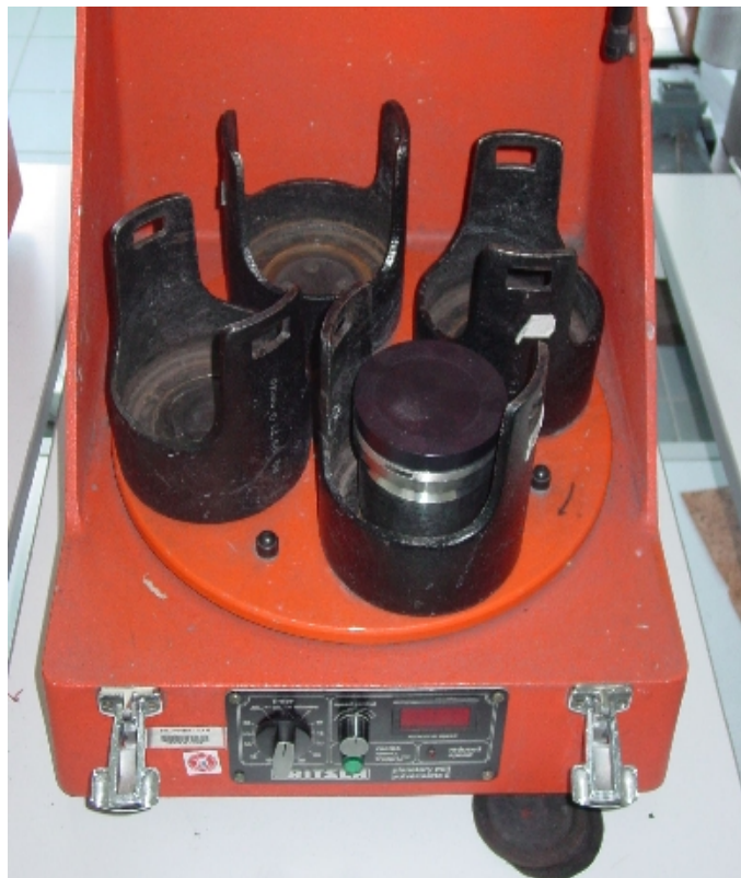
Figure 7: High energy ball milling with Pulverisette P5 (Fritsch, Germany), steel container (250 ml) filled with 100 balls (100 Cr6, 10mm diameter, 100 balls) stearic acid (0,5 or 1,0 Wt.%) rotation speed varied between 150 and 250 rpm 10 gram powder per milling vessel
