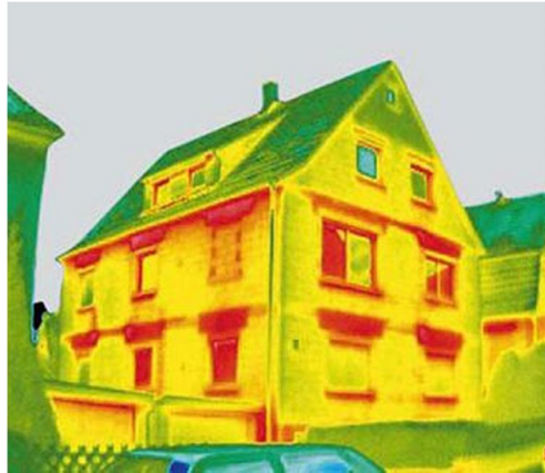
Figure 10: Thermal bridges location on thermal image of a building. [29]
