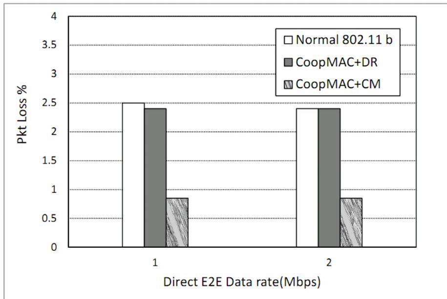
Figure 5.4 Packet loss percentage of UDP VOIP when using CM and DR as metric compared to 802.11b
