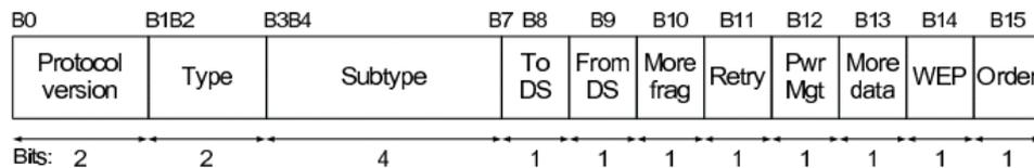
Figure I.8Format Frame Control
