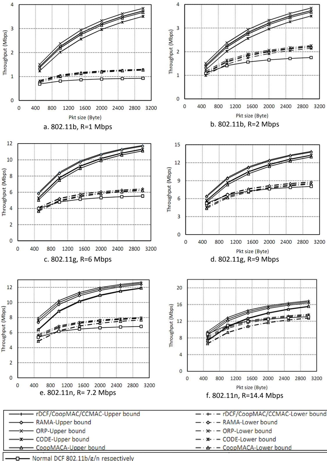
**Figure 4.6** Throughput performance bounds of Min-TX protocols in 4-way handshaking mode of DCF
