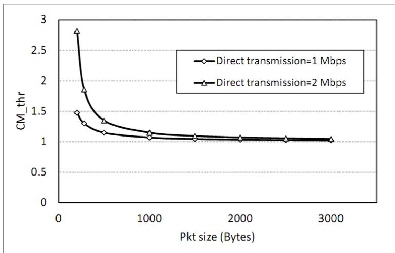
Figure 5.1 Threshold of CoopMetric versus the packet size for different direct data rates in IEEE 802.11b
