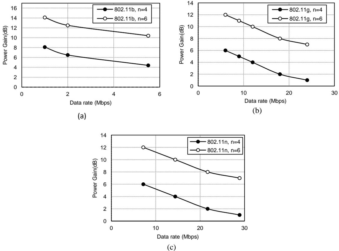
Figure 4.9 Power gain versus data rate and path loss coefficient ( $n$ ) in (a) 802.11b, (b) 802.11g and (c) 802.11n
