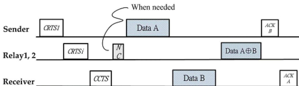
**Figure 3.3 Control and data packets in CODE protocol [21]**
