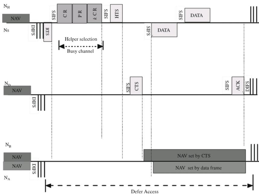
Figure 3.2 Time sequences of control and data packets in CoopMACA [20]
