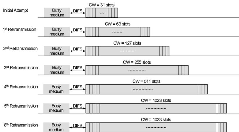
**Figure I.4 Minimum and maximum value of Contention Window**
