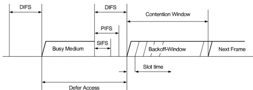
Figure I.3 Inter-frame Space in DCF mode
