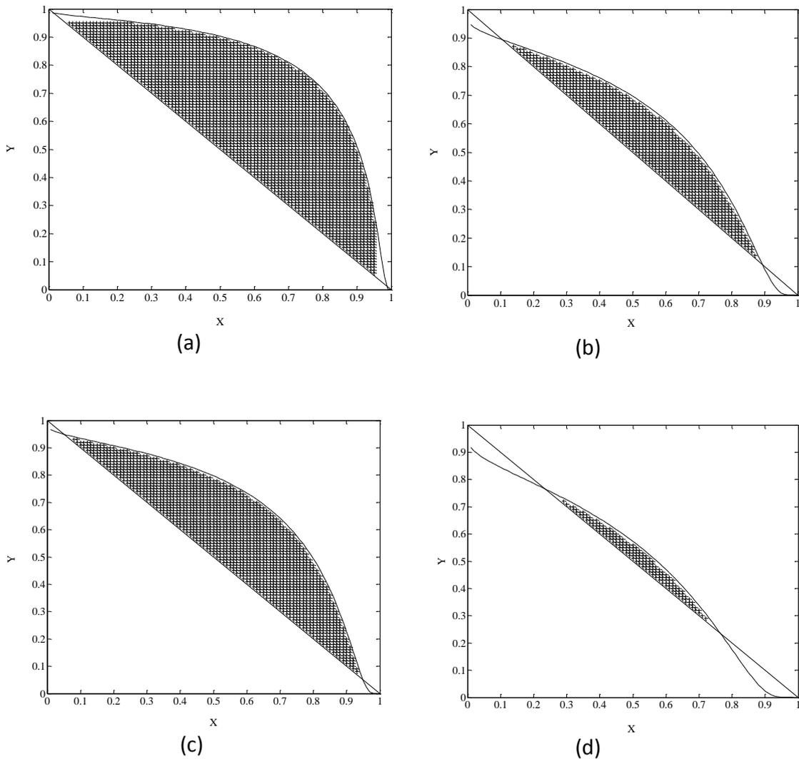
**Figure 4.3 Relay area of path loss coefficient ( $n=4$ ) and different SNR:(a) SNR=1, (b) SNR=3, (c) SNR=6 and (d) SNR=10**
