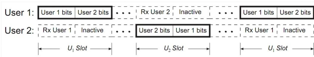
**Figure 2.4 Coded cooperation implementation for a system using TDMA [52].**
