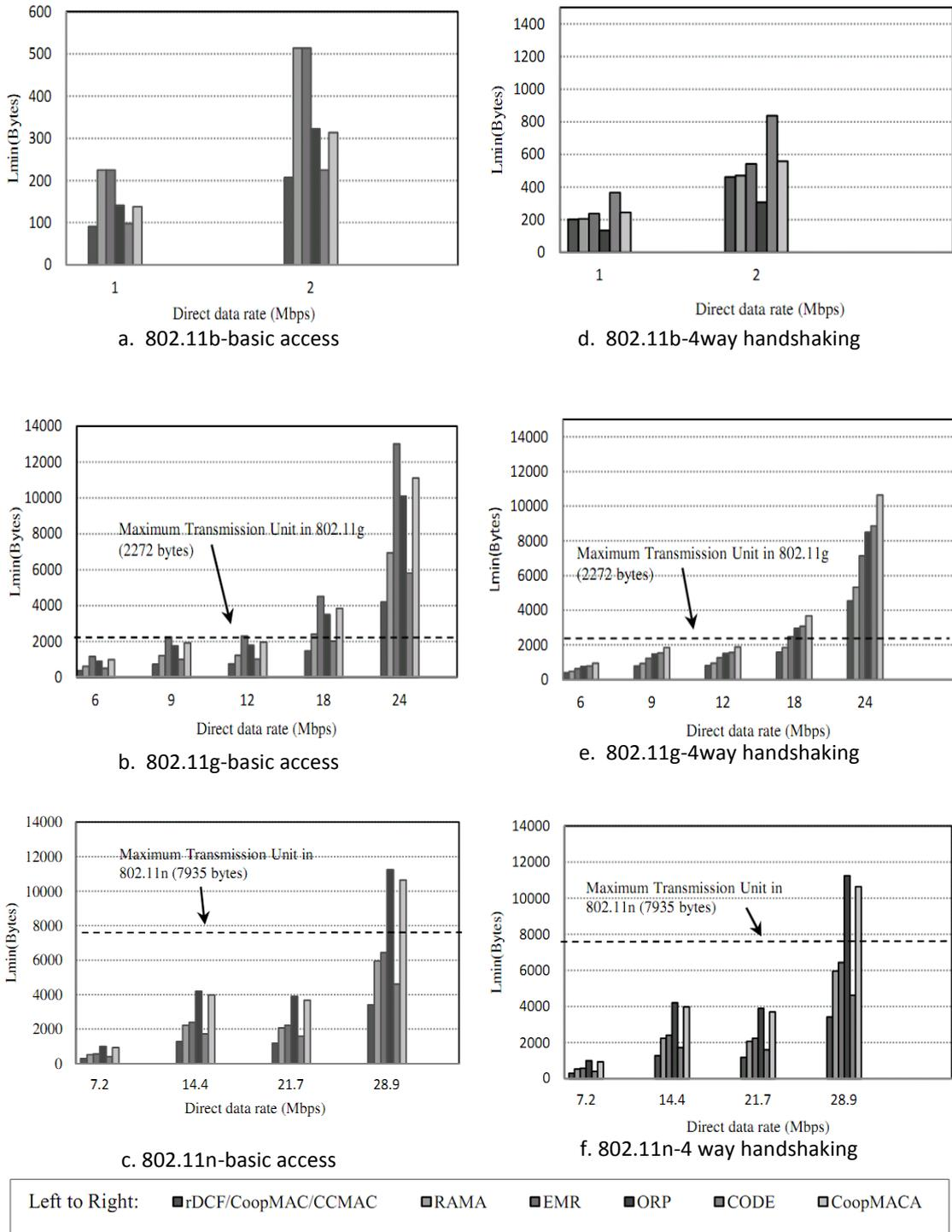
**Figure 4.7 Lower bound of data packet size of Min-TX protocols in basic access mode (a, b, c) and 4-way handshaking mode (d, e, f)**
