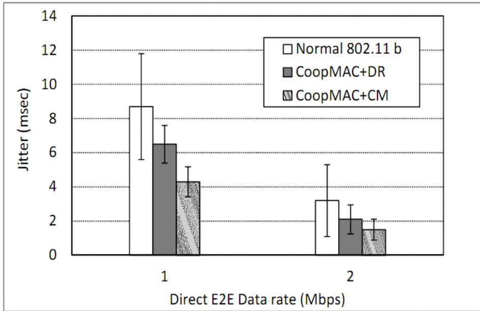
Figure 5.3 Jitter value of UDP VOIP when using CM and DR as metric compared to 802.11b
