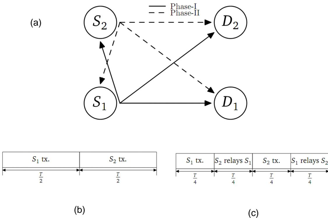
**Figure 2.3 (a) Simple TDMA based cooperation: (b) TDMA in non-cooperation mode (c) TDMA in cooperation mode**
