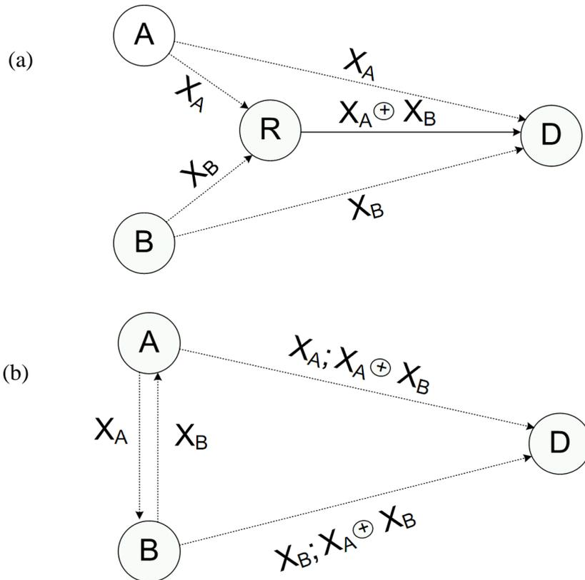
Figure 2.5 Cooperative communication with network coding
