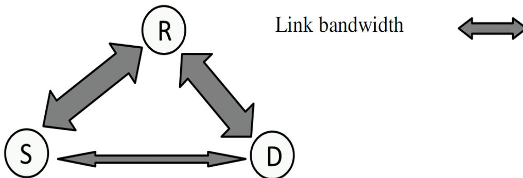
**Figure 2.2 Relay node as a repeater for cooperation at upper layers. (Width of arrows illustrate practical link bandwidth)**
