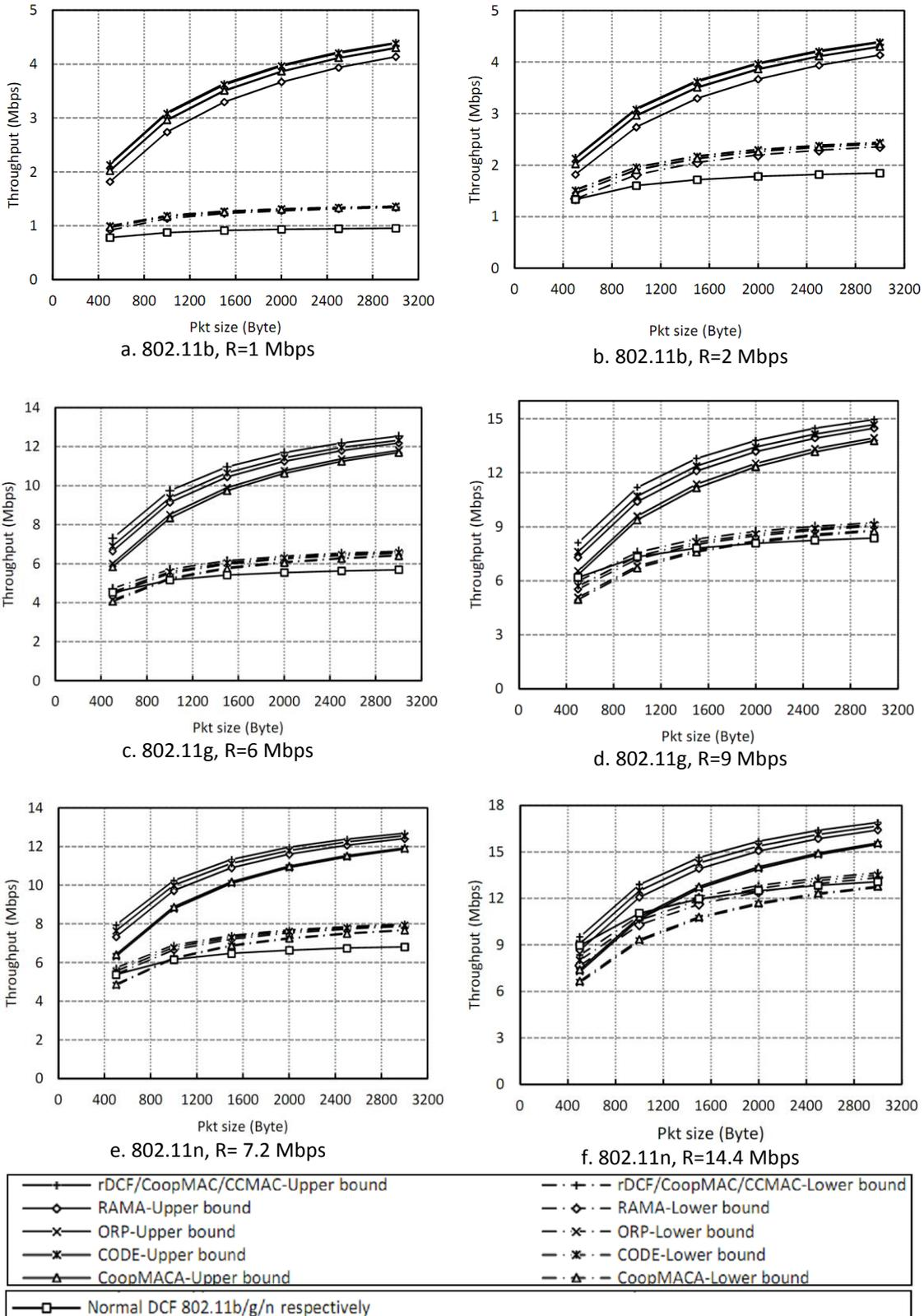
Figure 4.5 Throughput performance bounds of Min-TX protocols in basic access mode of DCF
