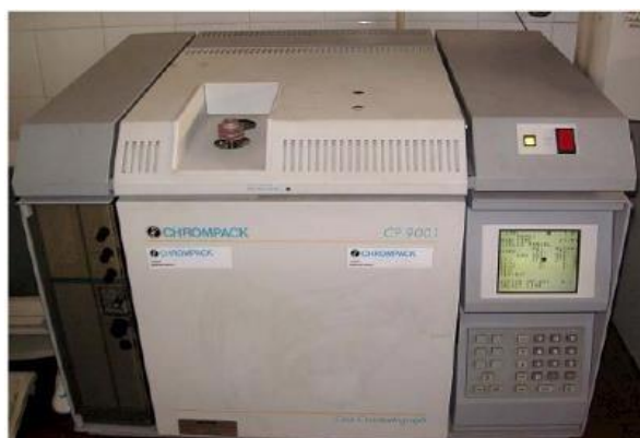
Figure 7 - Chromatograph (Chrompack brand, model CP9001).
