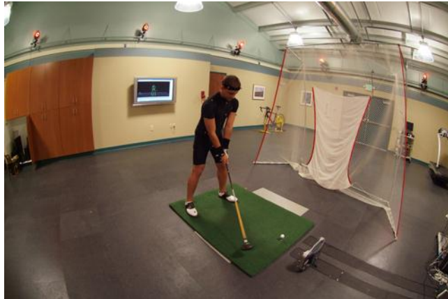
Figure 15 - Vicon motion capture system used in the kinematic analysis of the golf swing [81].
