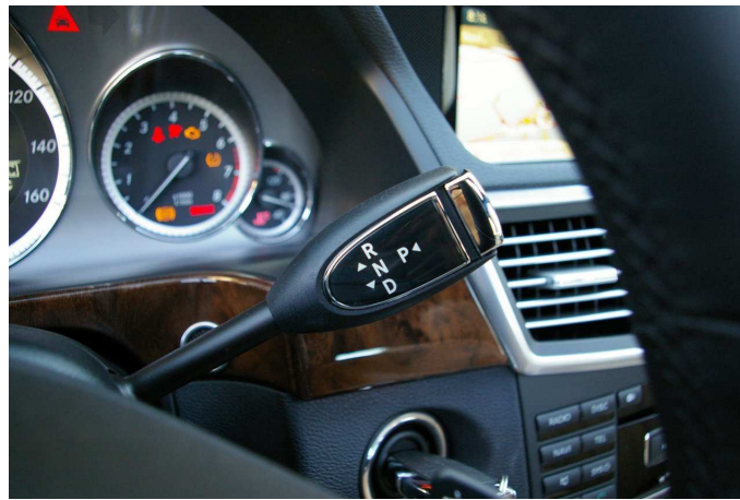
Figure 1.7: Steering column automatic mode selector lever from a 2010 Mercedes-Benz E350, with the four common modes: R, N D and P [7].
