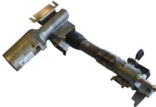
Figure 1.5: AtlasCar electrically controlled steering column.
