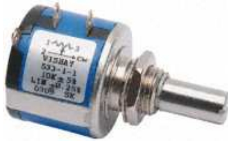
Figure 2.5: Vishay Spectrol Multiturn Wirewound Potentiometer [14]
