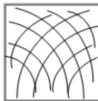
Figure 10 - Simplified representation of the stainless steel sample aspect after the grinding treatment.
