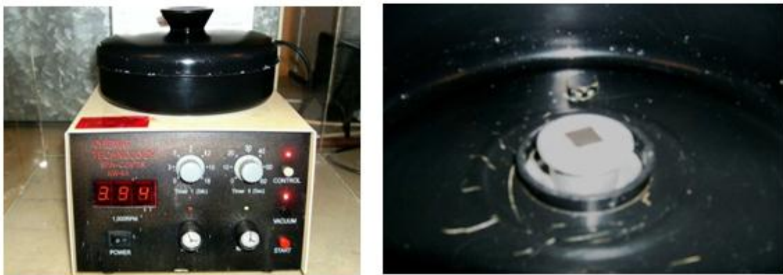
Figure 11 - Outer side and inner side of the spin-coater used in this work.
