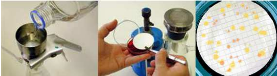
Figure 1.7. Filtration of peptone water through a Millipore membrane and microorganism's growth in Petri dishes during the incubation period.
