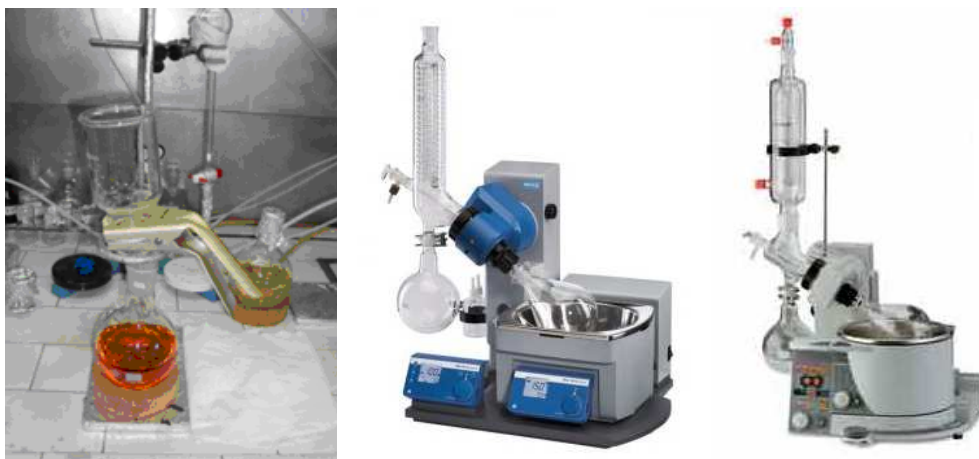
Figure 1.22. Filtration of the organic extracts and concentration of the solvent in a rotary evaporator (IKA HB 10 basic and Laborota 4002 – Digital, respectively).
