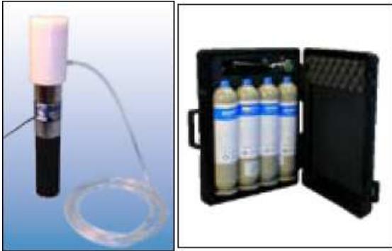
Figure 1.5. Gas calibration hood and certified cylinders used with the air quality monitor.
