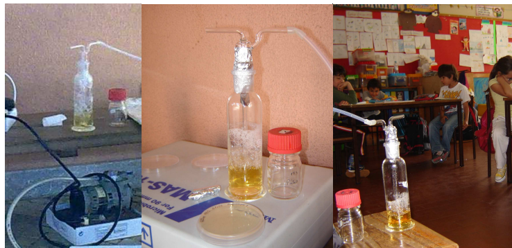
Figure 1.6. Liquid impinger sampling in classroom and at playground.
