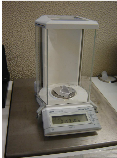
Figure 1.14. Filter loaded with PM 10 being weighted in the microbalance.
