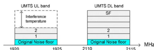
Figure 1: UMTS FDD spectrum bands with asymmetric load
