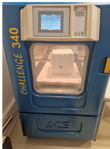
Figure 4.16: Sub zero temperature test.
