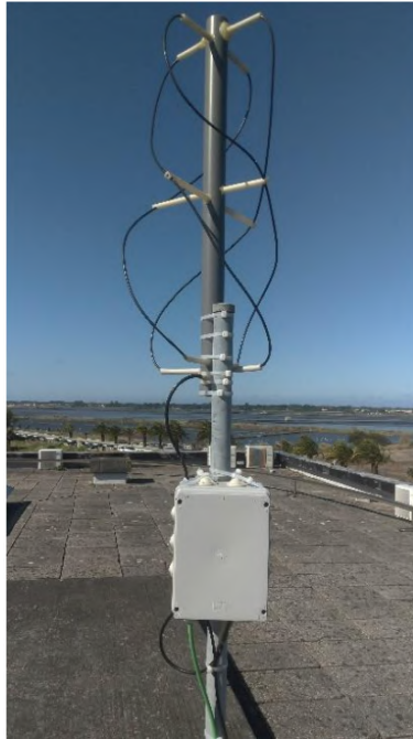
Figure 3.5: Projected NOAA satellites receiver setup [9].
