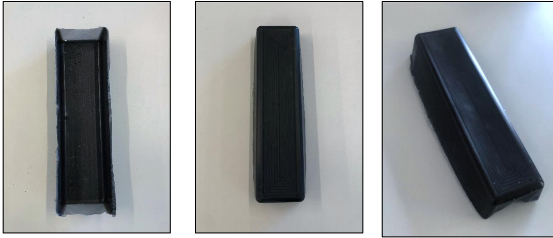
Figure 5.10. PA6/GN samples produced by T-RTM using 5 bar injection pressure.
