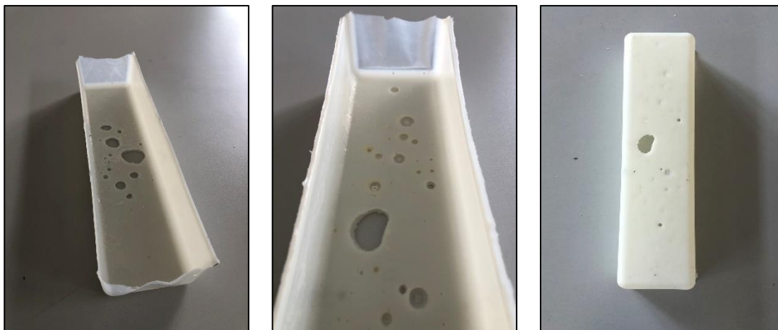
Figure 5.7. PA6 samples produced by T-RTM using 3 bar injection pressure.
