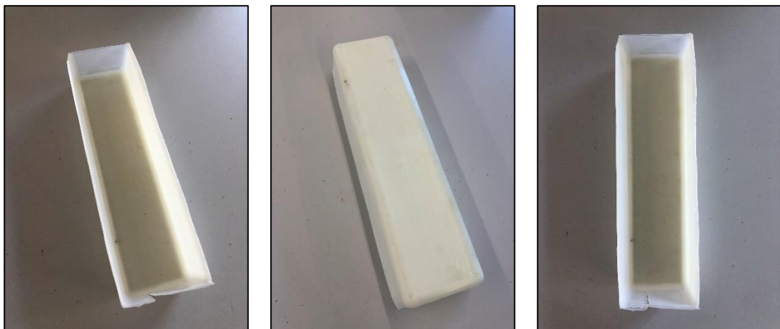
Figure 5.9. PA6 samples produced by T-RTM using 5 bar injection pressure.
