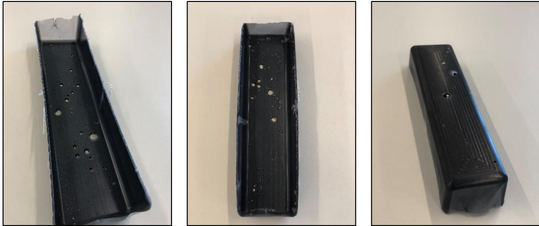
Figure 5.8. PA6/GN samples produced by T-RTM using 3 bar injection pressure.
