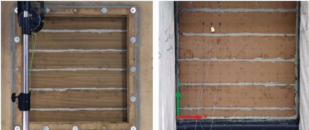
Figure 2.15: WPC view from the reverberation (left) and hemi-anechoic chamber (right) [44].
