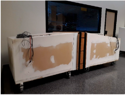
(a) Small scale reverberation chambers [19].
