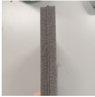
Figure 5.2: Bitumen heavy layer within the PUR foam.
