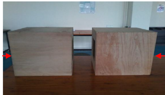
(b) Small scale reverberation chambers for testing fiber panels [20].
