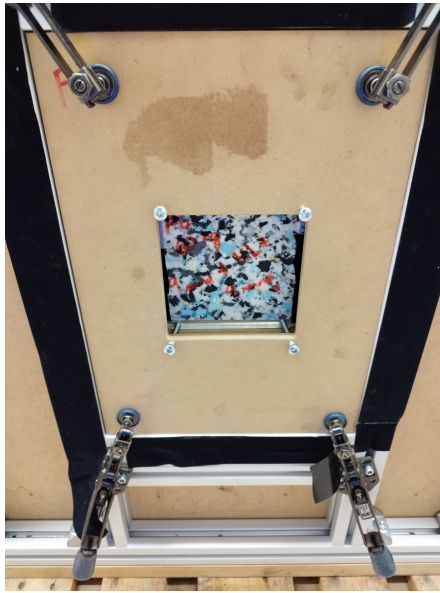
Figure 4.5: Sample holder in the reverberation chamber.
