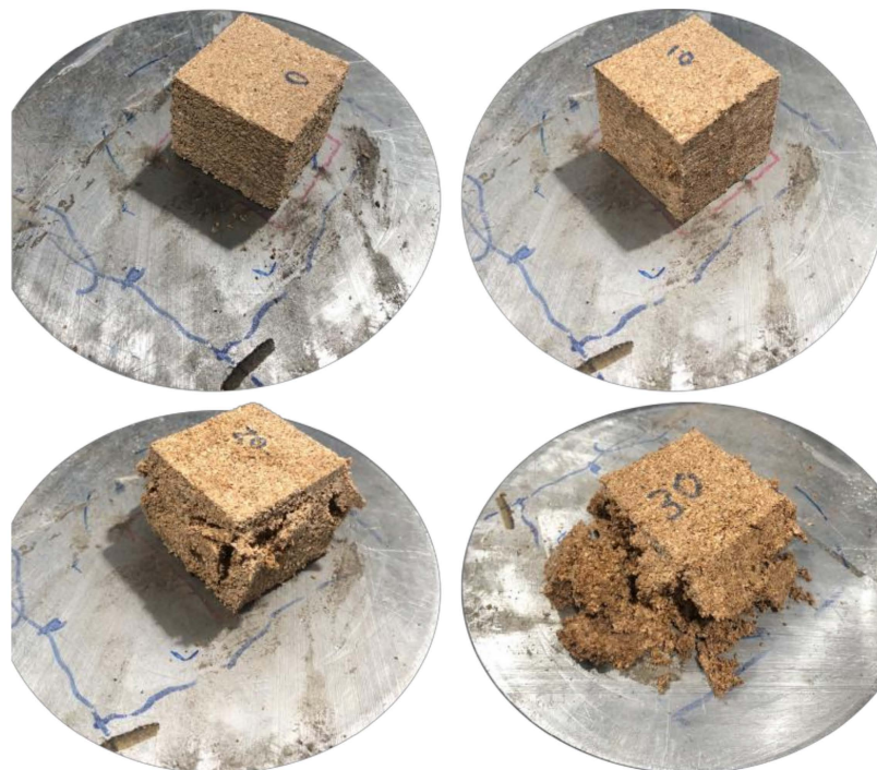
Figure 11. Samples after impact tests with the respective percentage indication of STF.
