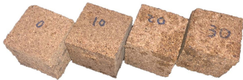
Figure 6. Samples were prepared with 0, 10, 20, and 30 wt.% of STF fluid.
