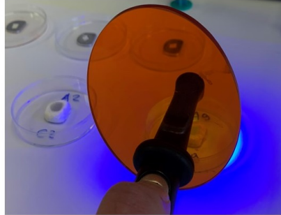
Figure 5.37: Crosslinking of the AG+Col-MA hydrogel with the UV light
