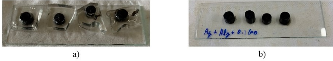
Figure 5.32: Hydrogel samples preparation. On the left side a), the hydrogel was poured into the moulds. On the right side b), the hydrogel samples after extraction from the moulds.
