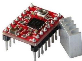
Figura 33 – Driver A4988 (PTRobotics, 2023)
