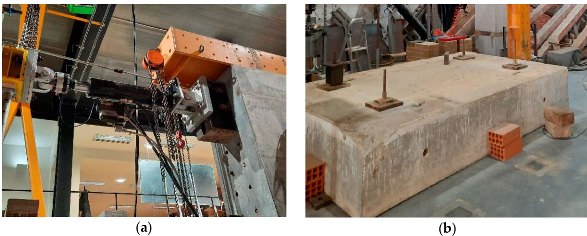
Figure 7. (a) Servo-actuator connection to the reaction wall; (b) fixing the footing on the reaction slab.
