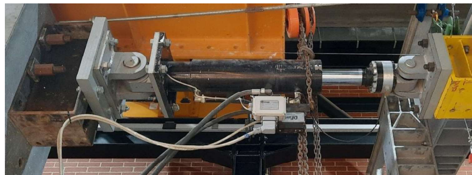
Figure 9. Servo-actuator with 200 kN of capacity and 400 mm stroke.
