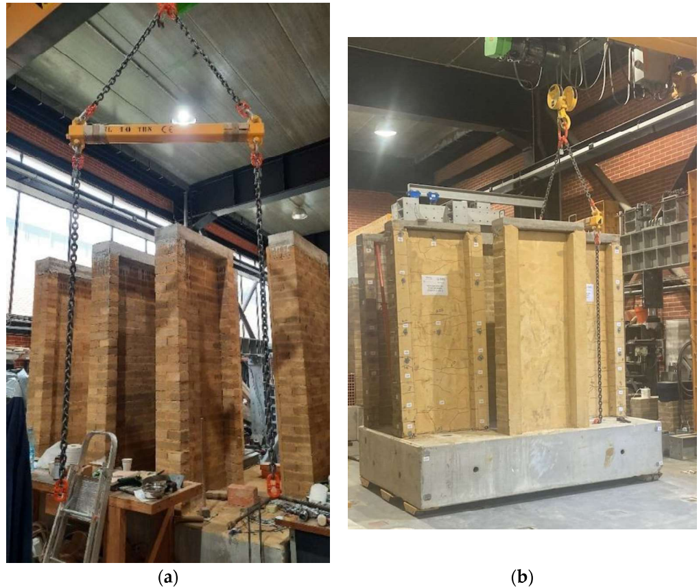
Figure 17. (a) Load spreader assembly. (b) Movement of the footing with specimens, with the help of roller skids, load spreader assembly, and overhead crane.
