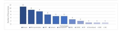
Figure 3: Technologies applied in bicycle warning systems (@authors).
