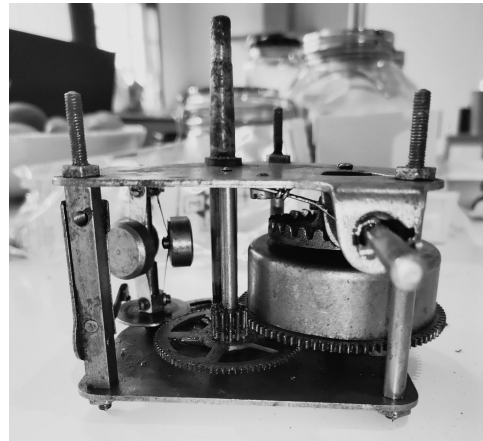
Fig. 2. The engine of a 1924 Pathé gramophone. Photograph taken by the author. Hidden inside a gramophone for reading shellac records was a wind-up motor with enough strength to keep the record at a constant speed of 78 r.p.m. during a reading that lasted about 3 minutes. The string was given by hand before each reading and sometimes required significant force by the operator.
