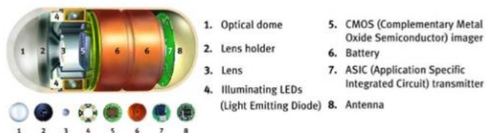
Figure 2.2 Example of an Endoscopy Capsule and respective components [7].
