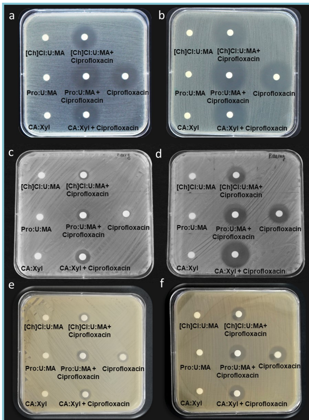
Figure 21. Antimicrobial susceptibility to ciprofloxacin formulated in DES aqueous solutions. Representative inhibition zone assay on cultures using disks impregnated with ciprofloxacin's aqueous solutions with [Ch]Cl:U:MA, Pro:U:MA, CA:Xyl on TSA plates. (a) and (b) for E. coli ATCC-25922, the antibiotic was tested at 0.5 (a) and 5.0 (b) \mu\text{g}\cdot\text{mL}^{-1} , respectively. (c) and (d) show the representative inhibition zone assays on P. aeruginosa ATCC-27853 cultures using disks impregnated with ciprofloxacin's formulations with the same DES in the same concentrations. (e) and (f) demonstrate the antimicrobial susceptibility of S. aureus ATCC 6538 to these solutions with the antibiotic at concentrations of 5.0 (e) and 10 (f) \mu\text{g}\cdot\text{mL}^{-1} , respectively. Ciprofloxacin in water and the DES aqueous solutions (without ciprofloxacin) were evaluated in the same concentrations.
