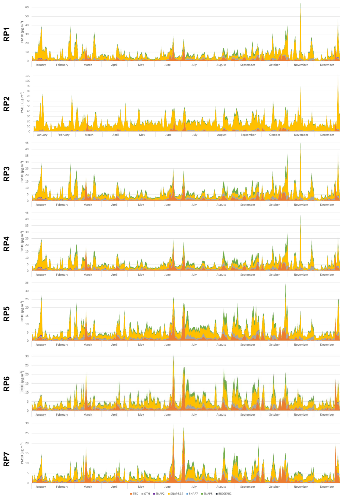
Figure 5.14. Daily contribution of each source sector for PM 10 concentration, in \mu\text{g}\cdot\text{m}^{-3} , for the medium-term future climate (2055), for each receptor point.
