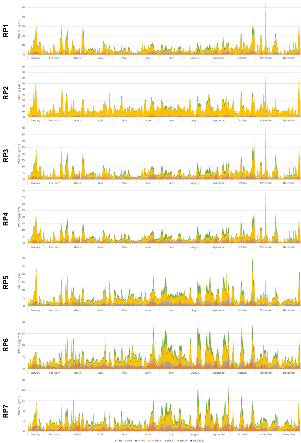
Figure 5.12. Daily contribution of each source sector for PM 2.5 concentration, in \mu\text{g}\cdot\text{m}^{-3} , for the medium-term future climate (2055), for each receptor point.
