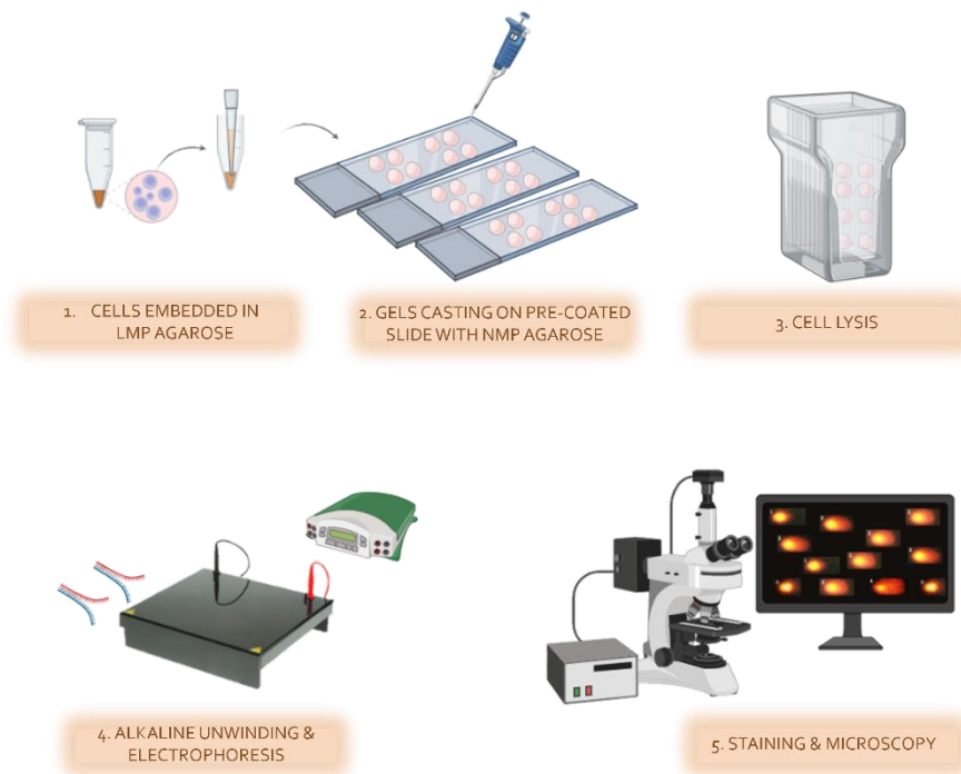
Fig. 2. Procedure of the comet assay. (1) microtube with cell suspension; (2) cell suspension embedded in agarose; (3) lysis (pH 10); (4) alkaline unwinding and electrophoresis (pH 13); (5) representation of stained comet-shaped nucleoids.
