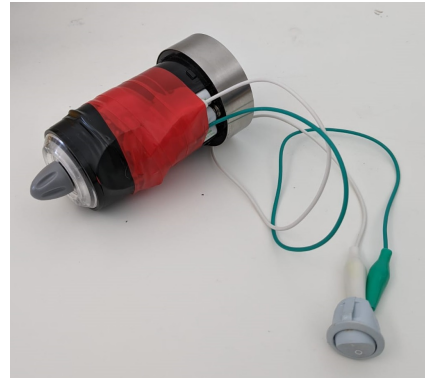
Figura 5.4: Pepper Mill adaptado com o switch On/Off.
