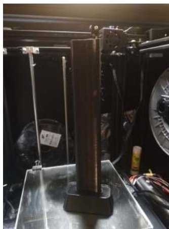
Figure 3.3: FDM printing process of slat and slat holder
