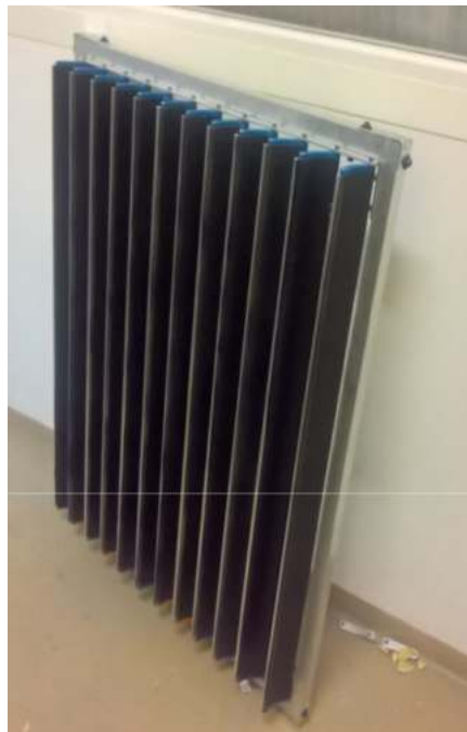
Figure 2.12: Vertical blinds filled with RT 28 [72]
