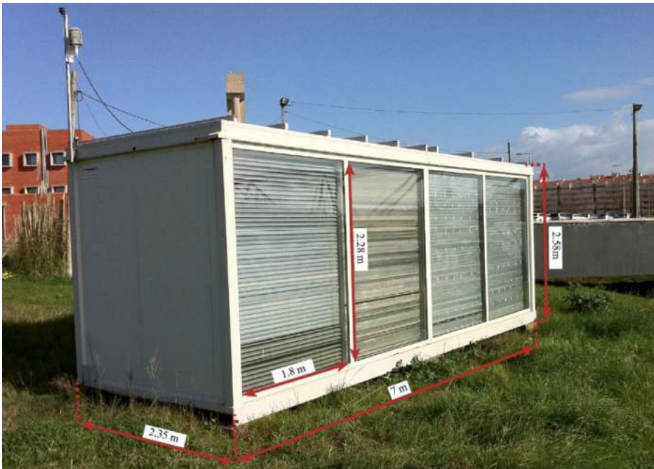
Figure 2.13: Window shutters filled with PCM RT28HC [73]
