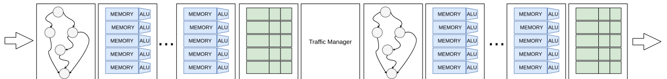
Figure 2.9: Portable Switch Architecture (PSA)
