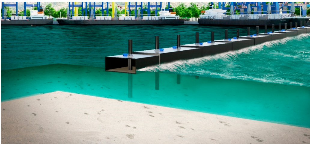
Figure 1.6. Illustration of a floating breakwater composed of heaving buoy WECs [51].
