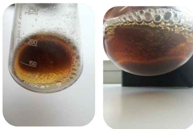
Figure 23: Flocculated S. stipitis in hydrolysate Erlenmeyer flask assays, at 18.5h of fermentation.
