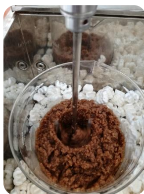
Figure 15: Unbleached Kraft pulp of E. globulus barks in citrate buffer solution during the hydrolysis process.
