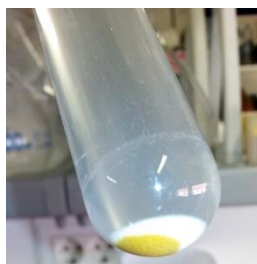
Figure 5.8. The photocatalyst aspect after 12 h of metoprolol photodegradation without stirring.
