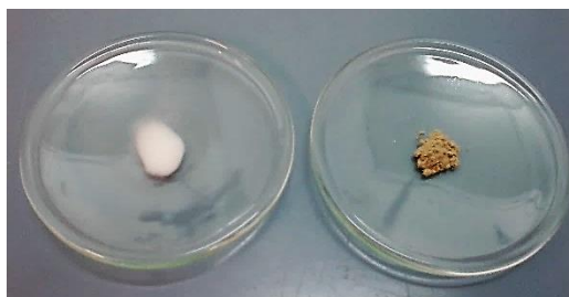
Figure 5.1. Appearance of the functionalized silica before the immobilization (left) and after the porphyrin immobilization (right).
