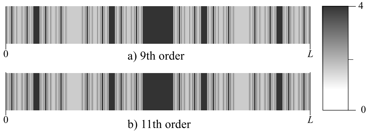
FIGURE 2.6: \varepsilon profile for the 9th and 11th order fractal MM by MPB. The black and gray color are \varepsilon_1 and \varepsilon_2 respectively.
