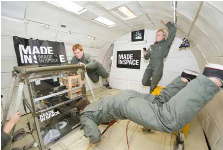
Figura 3.8 Teste à impressora 3D em ambiente de microgravidade ( Made in space; http://spaceflight101.com/iss/made-in-space-1st-iss-3d-printer/ )
