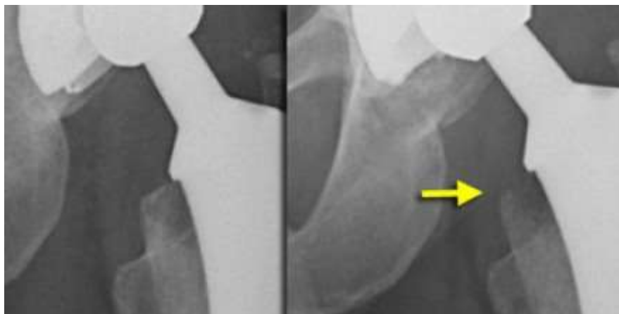
Figure 7: The effect of stress shielding on a hip stem. Left: Fixed prosthesis. Right: Loosened prosthesis [56]
