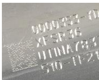
Riscagem (Technifor - Gravotech Marking, 2017a)
