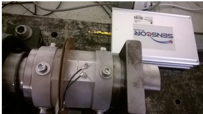
Figure 3.6: Load cell with the sensors attached and the RF Coupler positioned for measurement
