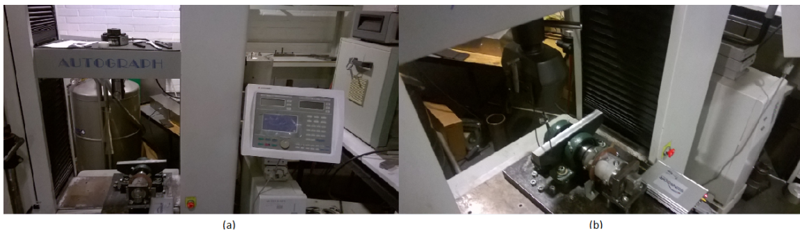
Figure 3.16: Experiments realized to obtain the SENSEOR SSE E015 and SSE E016 calibration curves: (a) Load cell torsional force applied in the downward direction (b) Load cell torsional force applied in the upward direction
