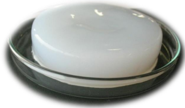
Figure 7 – Hydrated BC membrane grown under static conditions.
