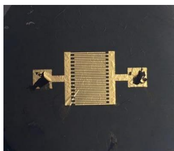
Fig.2-11, Failed etching process
