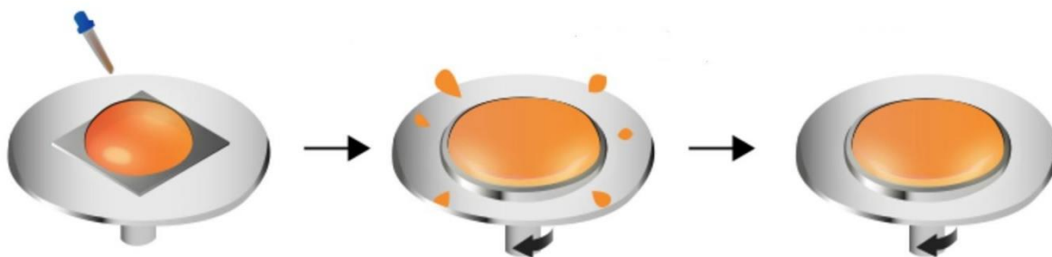
Fig.2-3. Spin coating process [1]
