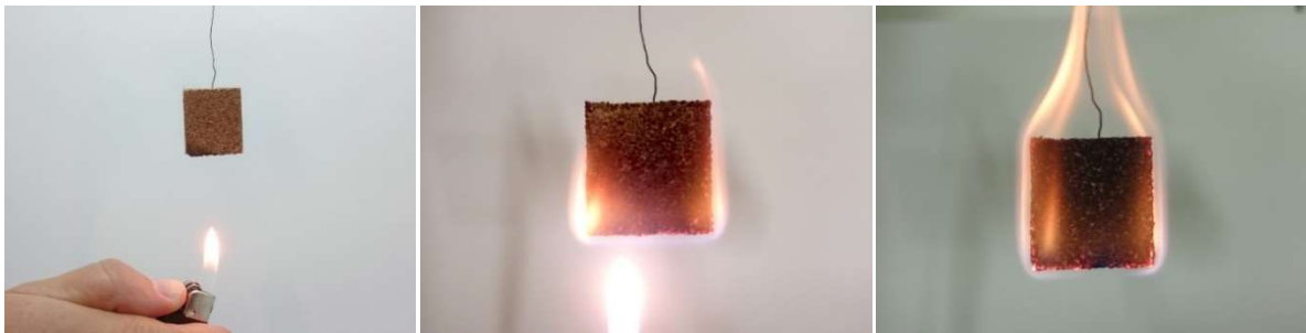
Figure 3.27: Burning test vertical sample set-up (sample with small grain (0.5-1mm), density ( 150 \text{ kg/m}^3 ) and 10 wt.% of flexible binder agent)
