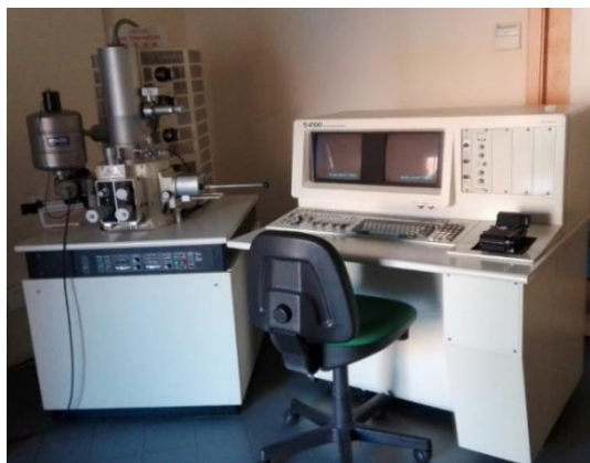
Figure 39. SEM used for observation of the spray dried granules morphology: HITACHI S-4100 microscope, available at University of Aveiro.
