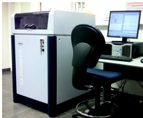
Figure 42. Equipment of X-ray Fluorescence Spectrometer (Bruker-AXS S4 Pioneer), available at INNOVNANO.
