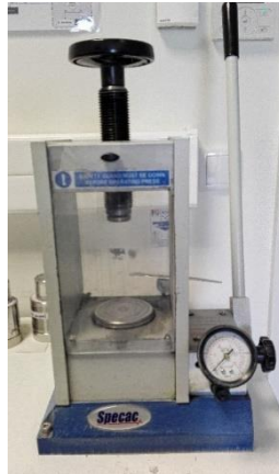
Figure 34. Specac's Laboratory Hydraulic Press, available at INNOVNANO.
