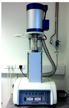
Figure 43. Vertical dilatometer (Linseis L-75 Platinum Series), available at INNOVNANO.
