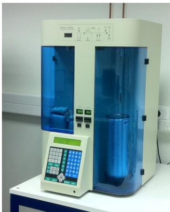
Figure 40. Specific surface area equipment: Nova 1000e Series System (Quantachrome) equipment, available at INNOVNANO.
