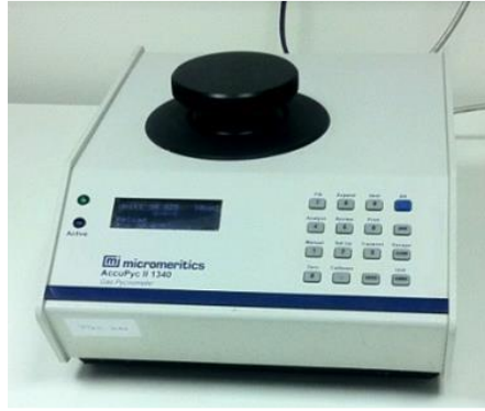
Figure 41. Helium pycnometer: AccuPyc II 1340 picnometer from Micrometrics, available at INNOVNANO.
