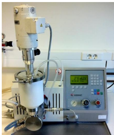
Figure 31. Micrometric bead mill Dispermat® SL12-nano, available at INNOVNANO.
