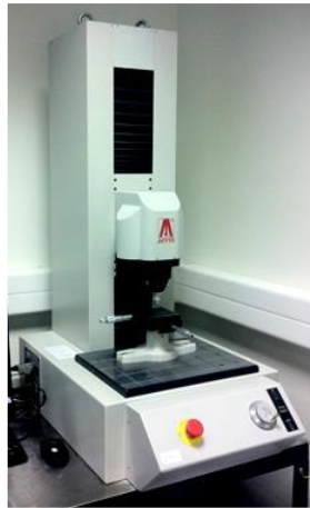
Figure 37. Vickers Hardness equipment: WIKI 100B Vickers Hardness Tester, available at INNOVNANO.
