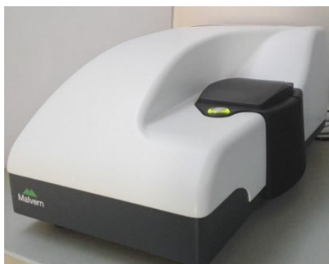
Figure 30. The measurements of zeta potential was performed on Zetasizer Nano ZS from Malvern, Available at the University of Aveiro.
