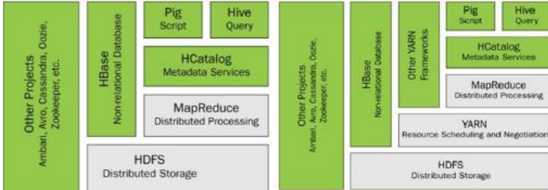
Figure 11 - Differences between prior Hadoop Version and Hadoop 2.0 using YARN[24]
