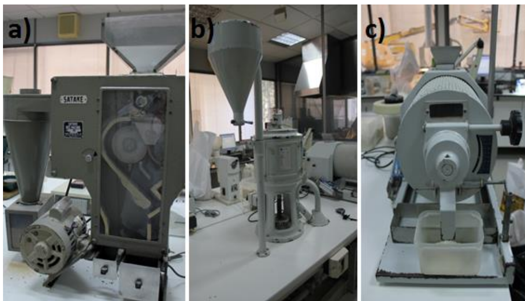
Figure 7 - Novarroz laboratory: hull removing (a) , milling (b) and separation of the whole rice grains and broken rice grains (c) .
