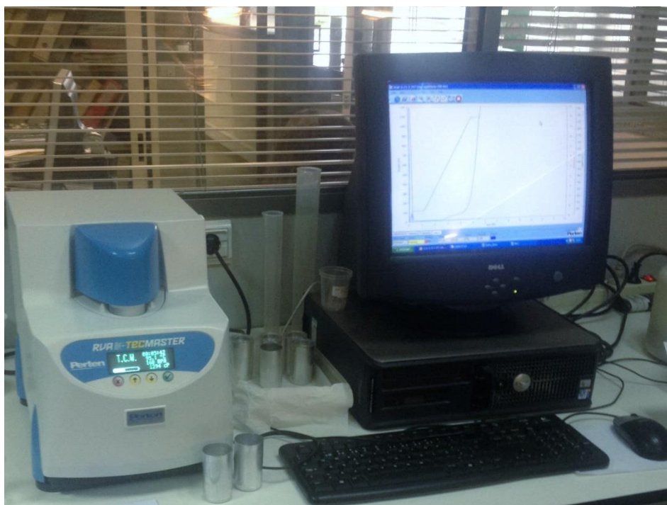
Figure 12 - Rapid Visco Analyser (RVA), model TecMaster , located in the laboratory of quality control of Novarroz.
