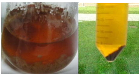
Figure 10 – Precipitate obtained after autoclaving the hydrolysate (left) and after centrifuging the previous solution (right).
